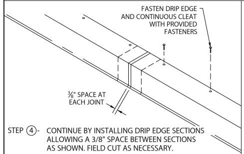
TYPICAL INSTALLATION SPLICE -**ROOFING** DRIP **MEMBRANE PLATE EDGE FASTENERS** (PROVIDED) CONTINUOUS CLEAT
