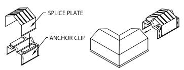
STEP 2 - MITER SPLICE PLATES & ANCHOR CLIPS POSITION THE SPLICE PLATE IN THE CENTER OF THE ANCHOR CLIP. INSTALL THE SPLICE PLATE AND ANCHOR CLIP ASSEMBLY INTO EACH END OF THE MITER AS SHOWN
