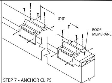
LOCATE AND FASTEN GALVANIZED ANCHOR CLIPS TO THE WALL AT 3'-0" O.C. WITH PROVIDED FASTENERS (SEE DETAIL A)
