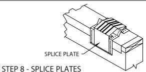
PLACE SPLICE PLATE ONTO ANCHOR CLIPS AT SPLICE JOINTS, 12'-0" O.C.
