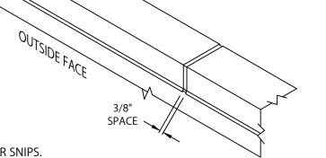
STEP 10 - COMPLETION CONTINUE INSTALLING COPING WITH A 3/8" SPACE AT SPLICE JOINTS TO ALLOW FOR THERMAL EXPANSION. FIELD CUT WHERE NECESSARY USING FINE TOOTH HACKSAW OR SNIPS. REMOVE PROTECTIVE FILM IMMEDIATELY.
