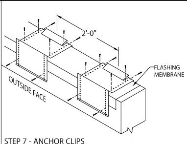
LOCATE AND FASTEN GALVANIZED ANCHOR CLIPS TO WALL AT 2'-0" CENTERS WITH PROVIDED FASTENERS FOR SUBSTRATE (SEE DETAIL A).
