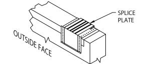
STEP 8 - SPLICE PLATES PLACE SPLICE PLATE ONTO ANCHOR CLIPS AT SPLICE JOINTS, 12'-0" O.C. NOTE: REMOVE RELEASE PAPER FROM SEALANT STRIPS.
