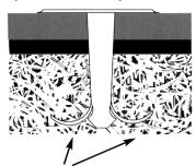
As locking staple is driven, its dual wire legs diverge anchoring the fastener in place.
