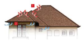
1. Stale air excapes through Cobra® Hip Vent (installed under cap shingles at the hips)
