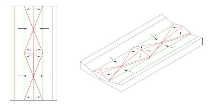
4-Way Slope Design; Optimized Performance, Direct Drainage
